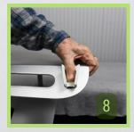
**8.** Peel protective paper from double sided foam tape on back of remote caddy and place on left side of computer tray. Press down with moderate pressure for ten seconds.
