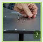
7. Finish tightening with short end of allen wrench until snug and then tighten an additional quarter turn.
