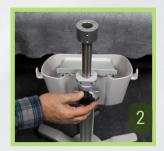
2. Turn the black plastic knob ½ turn counter-clockwise and fully extend the shaft.
