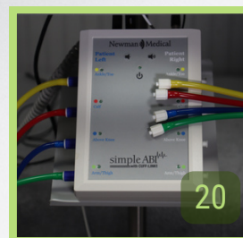
20. Locate the WHITE connector hoses for the right-side Cuff-Link ports.
